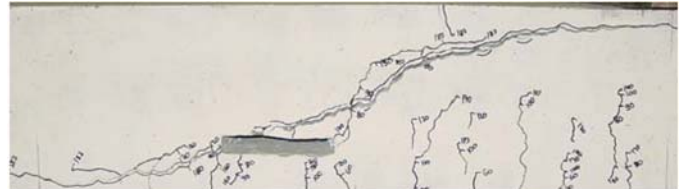
Picture 1-1: break pattern of a test specimen
