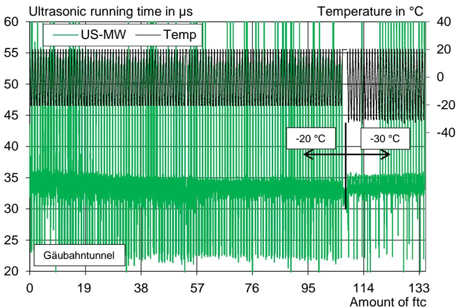
**Picture 2:** Ultrasonic running time of the concrete Gäubahntunnel during freezing cycles
