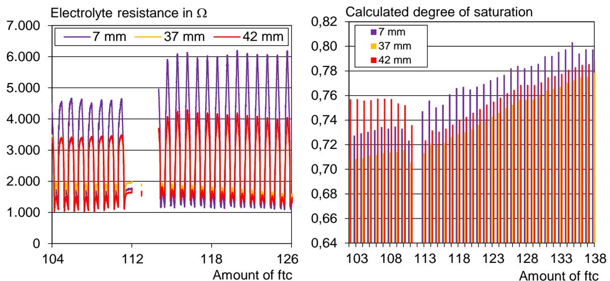
**Picture 5:** Freezing processes and calculated degrees of saturation at 20 °C of the concrete Gäubahntunnel at the time of lowering the minimum temperature
