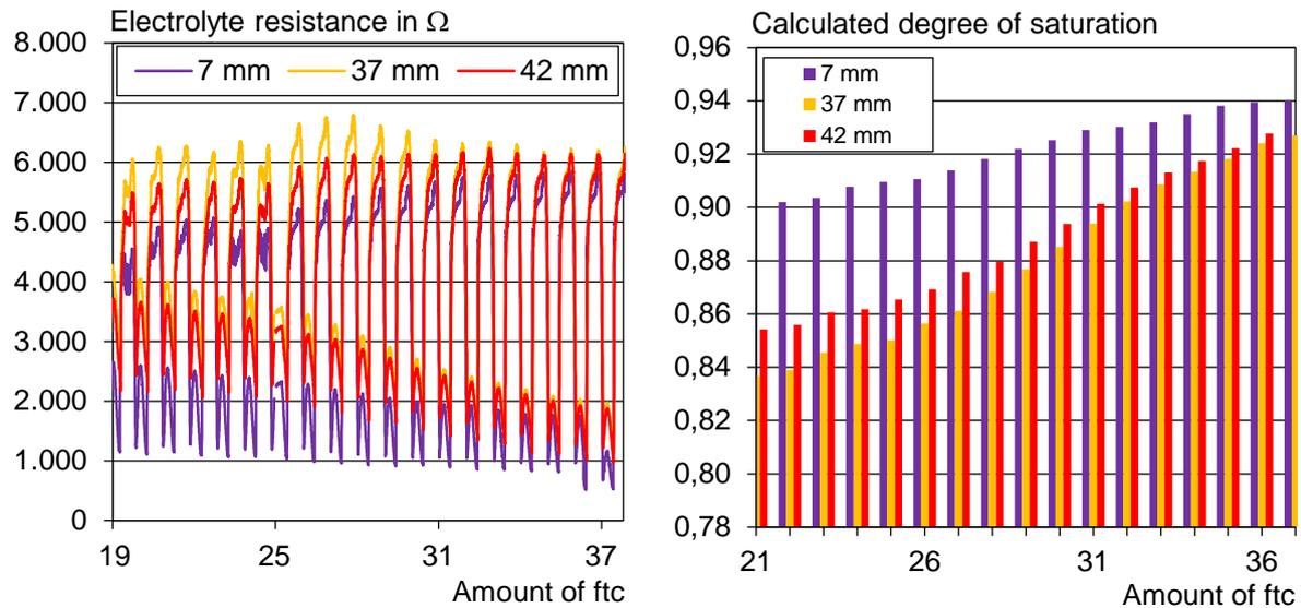
**Picture 4:** Freezing processes and calculated degrees of saturation at 20 °C of the concrete Hohenwarthe at the time of damage
