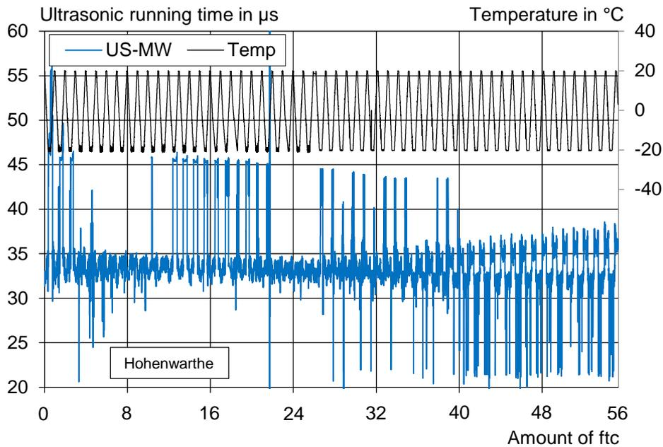
**Picture 1:** Ultrasonic running time of the concrete Hohenwarthe during freezing cycles
