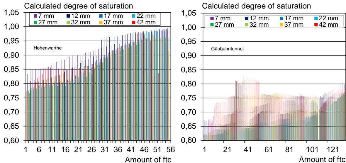
**Picture 3:** Calculated degrees of saturation of the concretes Hohenwarthe and Gäubahntunnel
