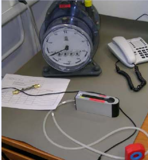
Control of air flow through all different types of sampling tubes received from the participants
