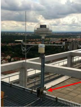
A photograph showing a pyranometer sensor mounted on a rooftop terrace. The sensor is a white dome-shaped device on a vertical pole. A red arrow points from the right side of the image towards the base of the sensor pole where it is secured to the roof structure. The background shows a cityscape under a cloudy sky. |
