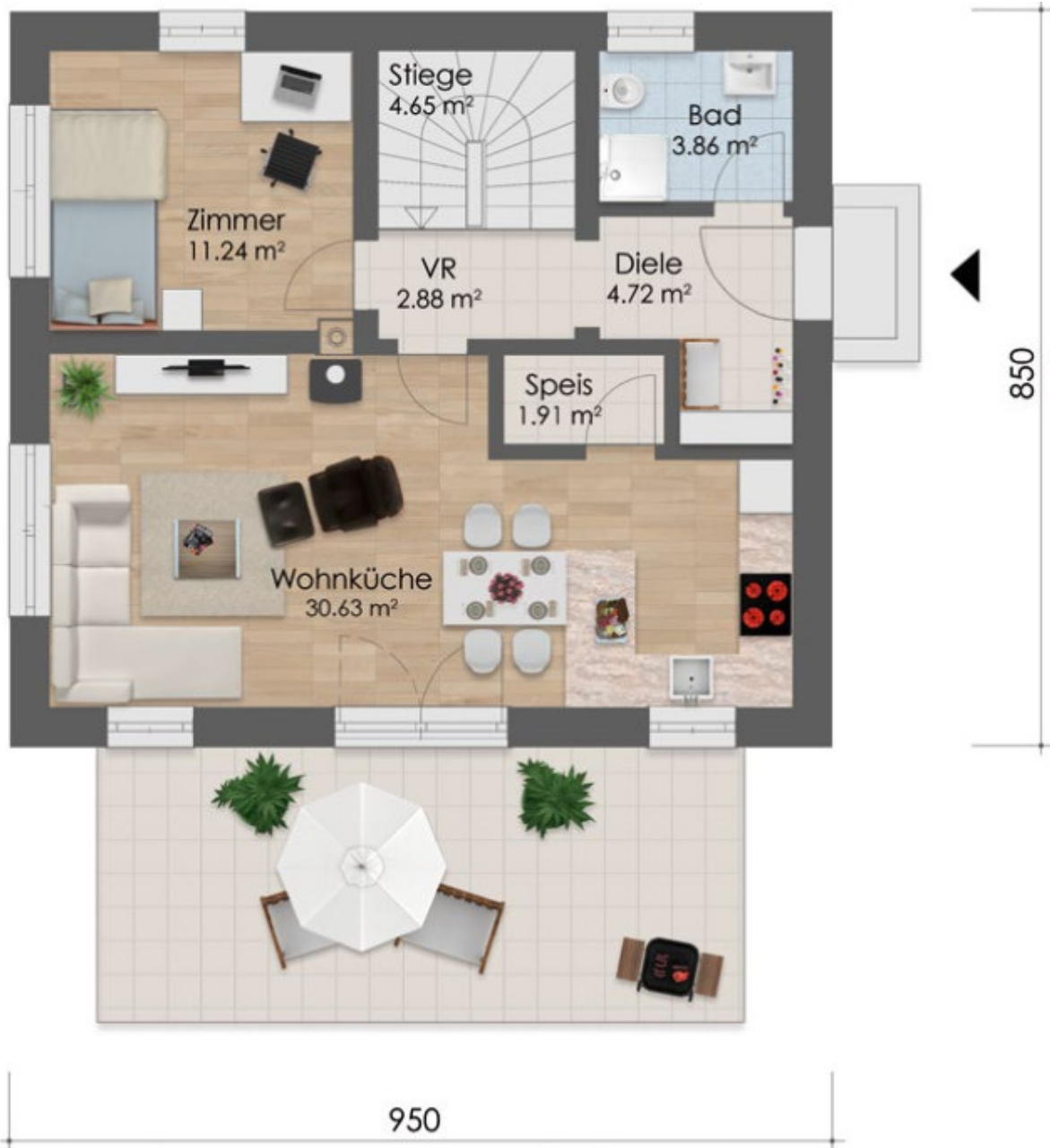
Figure 16-9: One family house, lightweight concrete, total area 120 m 2
