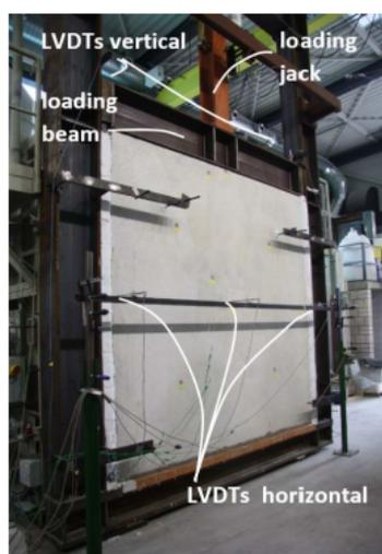
Figure 5. Loading setup for eccentrically loaded fire tests
