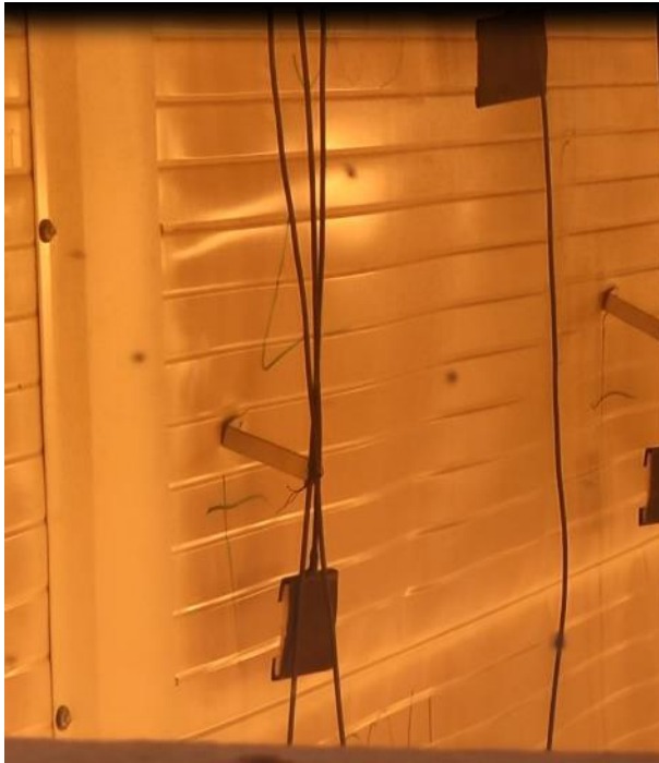
Abb. 6.8: Beulen Deckschicht innen (1')
