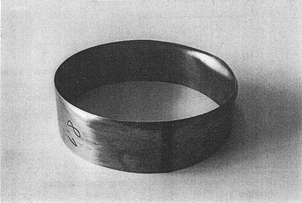
Fig. 8: Characteristic buckling shape in the elastic-plastic transition zone ( $r = 125 \text{ mm}$ ;  $t = 1 \text{ mm}$ )
