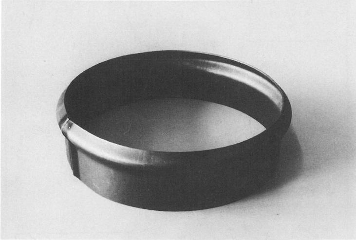
Fig. 7: Characteristic buckling shape in the fully plastic region
