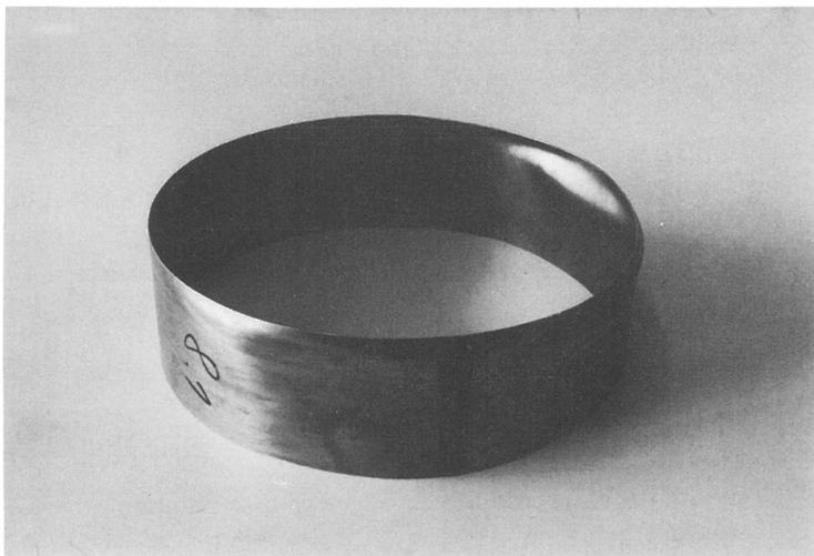
Fig. 8: Characteristic buckling shape in the elastic-plast: transition zone ( $r = 125 \text{ mm}$ ;  $t = 1 \text{ mm}$ )
